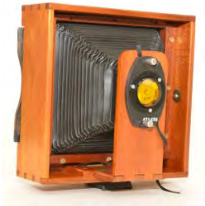
Fig. 8: 5" x 7" pinhole camera constructed from mahogany block given by Ian Hopkins
